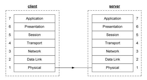
The data we want to communicate is generated in the application layer and then passed down the different layers. The client and server are connected on the physical layer by a medium, for example a cupper cable.
